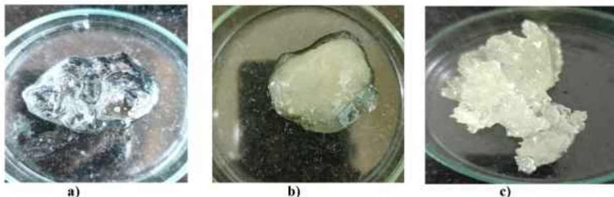
Fig. 8. Images of EVAM samples after 24 h absorption a) curing 1 h, b) curing 4 h and c) curing 24 h.
