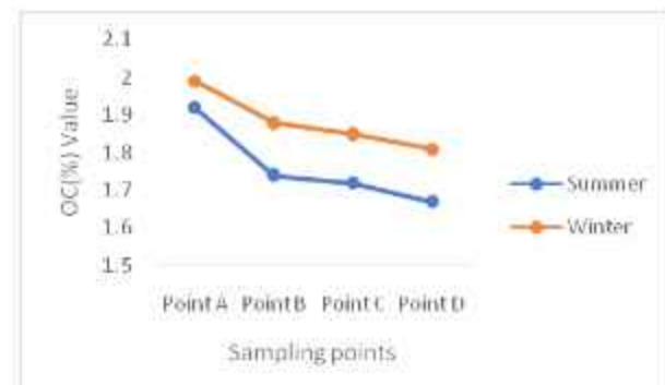
Fig. 3. Organic carbon content of crude oil contaminated soil in both summer and winter season
